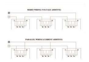
the positive terminal of one module to the negative of the next module. Figure shows modules connected in series .
